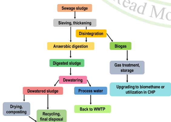
Diagrammatic sketch of sewage sludge production and possible resource recovery
